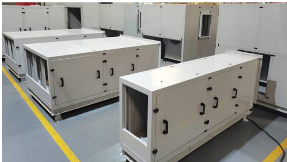
A well-stocked warehouse (top) has everything needed to manufacture a host of different products from fans to control boxes. Ecology unit cases (above) await installation of the electrostatic precipitators, filters and fans before delivery to the job site.
