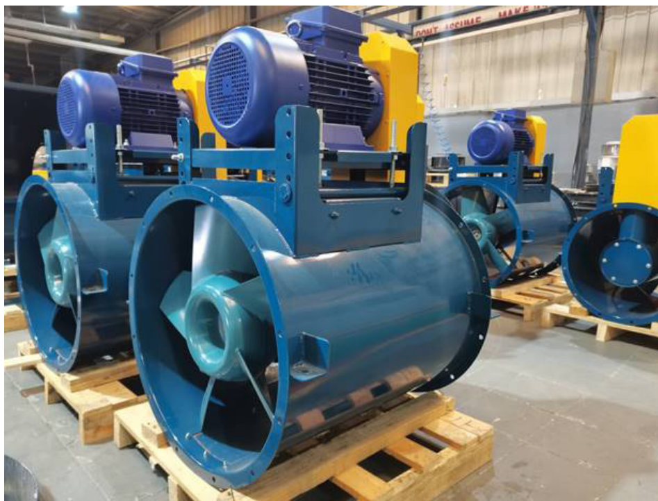
Energy Twin City fans (above) are palletted and prepared for final shipping. Through the joint venture, Energy Twin City can produce a wide range of Twin City fans. Along with HVAC products, Energy Industrial designs and manufactures electrical control boxes for use in commercial and industrial applications. The boxes at left are awaiting their internal wiring.
